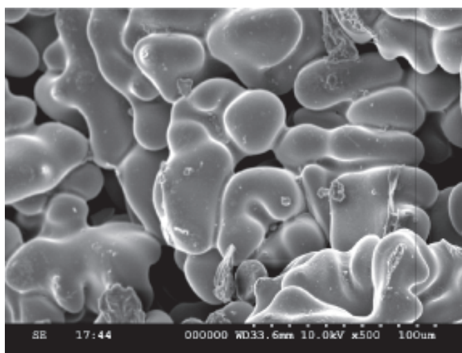
Fig. 10 : SEM Micrograph of the aged composites showing the adhesion of the precipitate to the particle
