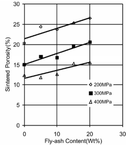
Figure 20: Effect of Fly-ash Content on Sintered Porosity of Al-15wt% Pb/fly-ash Composites Sintered at 530 °C
