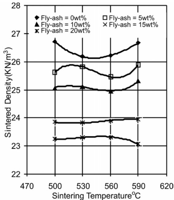
Figure 14: Effect of Sintering Temperature on Sintered Density of Al-15wt% Pb/fly-ash Composites Compacted at 400MPa
