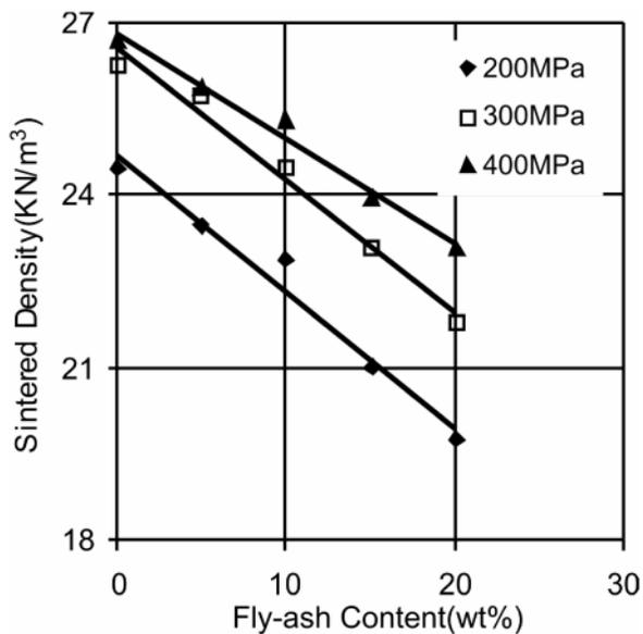
Figure 11: Effect of Fly-ash Content on Sintered Density for Al-15wt% Pb/fly-ash Composites Sintered at 590 °C
