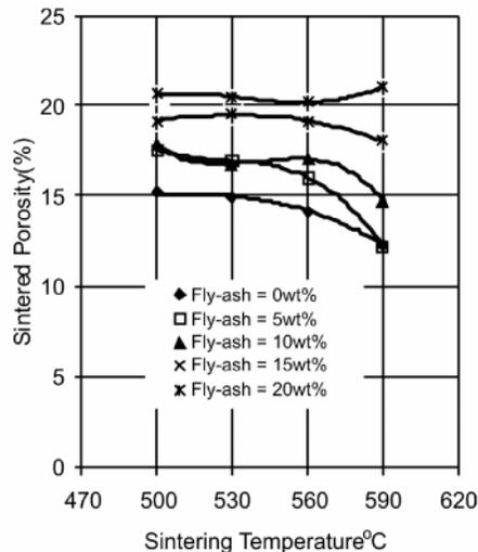
Figure 24: Effect of Sintering Temperature on Sintered Porosity of Al-15wt% Pb/fly-ash Composites Compacted at 300MPa
