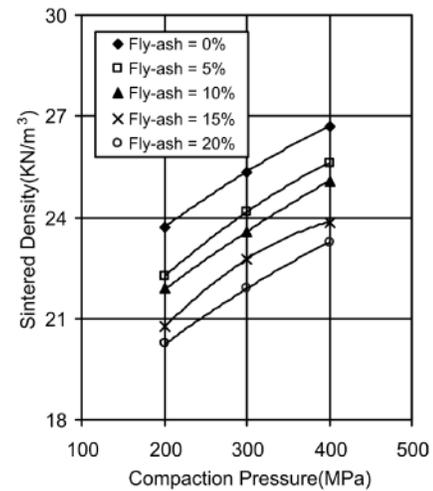
Figure 1: Effect of Compaction Pressure on Sintered Density for Al-15wt% Pb with 0 to 20wt% Fly Ash Sintered at 500 °C
