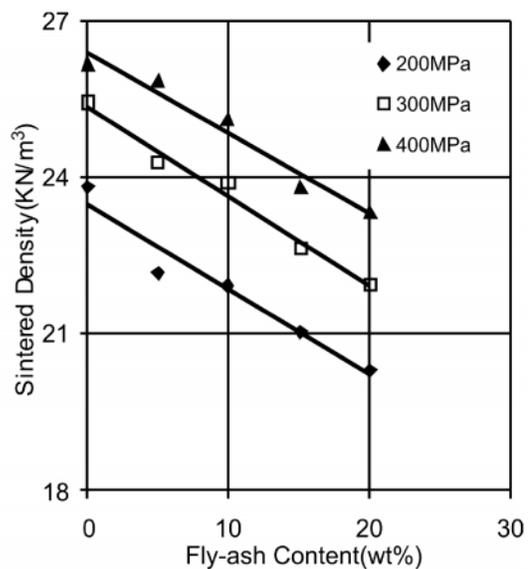
Figure 9: Effect of Fly-ash Content on Sintered Density for Al-15wt% Pb/fly-ash Composites Sintered at 530 °C
