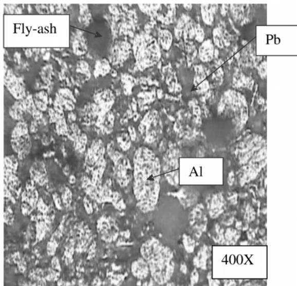
Figure 6: Microphotograph of Al-15wt% Pb/5wt% Fly-ash Composite Compacted at 300MPa and Sintered at 500 °C
