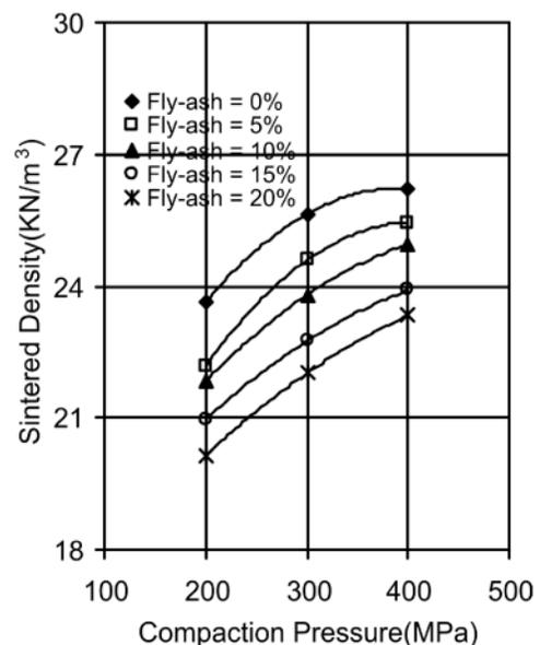
Figure 3: Effect of Compaction Pressure on Sintered Density for Al-15wt% Pb with 0 to 20wt% Fly Ash Sintered at 560 °C
