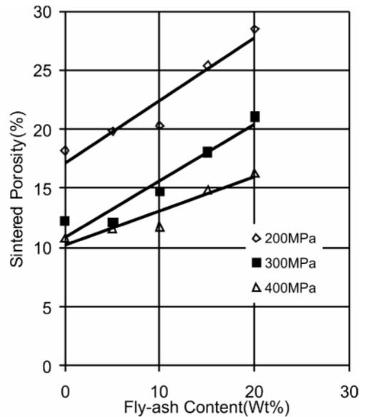
Figure 22: Effect of Fly-ash Content on Sintered Porosity of Al-15wt% Pb/fly-ash Composites Sintered at 590 °C
