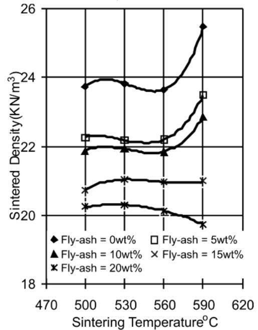
Figure 12: Effect of Sintering Temperature on Sintered Density of Al-15wt% Pb/fly-ash Composites Compacted at 200MPa
