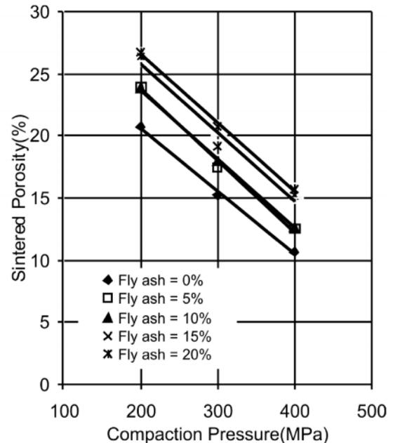
Figure 15: Effect of Compaction Pressure on Sintered Porosity of Al-15wt% Pb/fly-ash Composites Sintered at 500 °C
