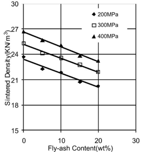
Figure 8: Effect of Fly-ash Content on Sintered Density for Al-15wt% Pb/fly-ash Composites Sintered at 500 °C
