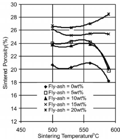
Figure 23: Effect of Sintering Temperature on Sintered Porosity of Al-15wt% Pb/fly-ash Composites Compacted at 200MPa
