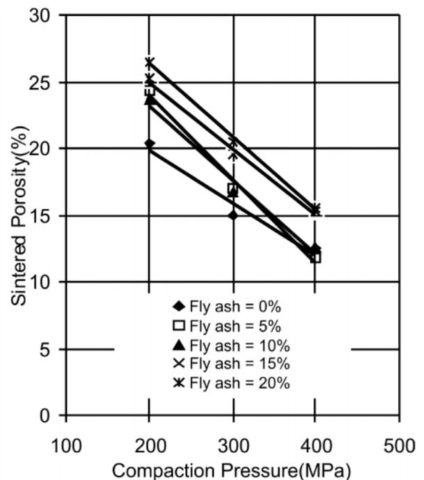
Figure 16: Effect of Compaction Pressure on Sintered Porosity of Al-15wt% Pb/fly-ash Composites Sintered at 530 °C
