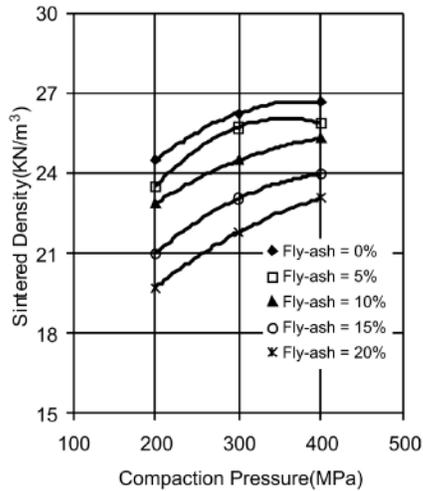
Figure 4: Effect of Compaction Pressure on Sintered Density for Al-15wt% Pb with 0 to 20wt% Fly Ash Sintered at 590 °C
