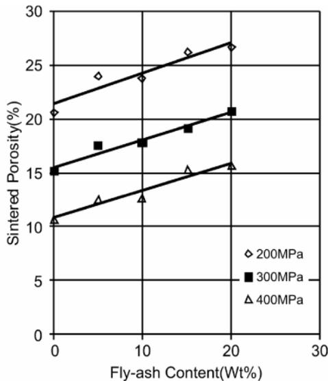
Figure 19: Effect of Fly-ash Content on Sintered Porosity of Al-15wt% Pb/fly-ash Composites Sintered at 500 °C
