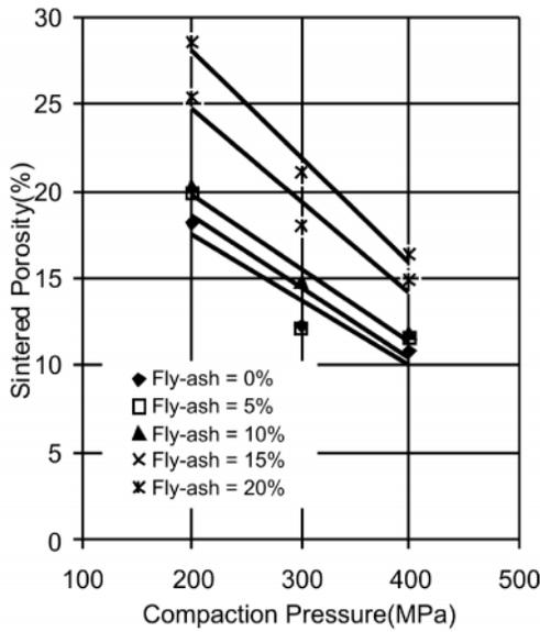
Figure 18: Effect of Compaction Pressure on Sintered Porosity of Al-15wt% Pb/fly-ash Composites Sintered at 590 °C
