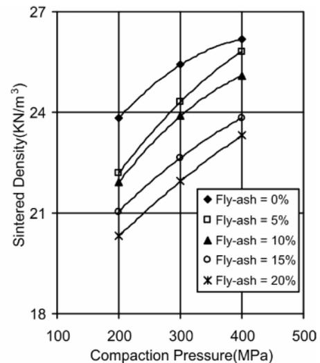
Figure 2: Effect of Compaction Pressure on Sintered Density for Al-15wt% Pb with 0 to 20wt% Fly Ash Sintered at 530 °C
