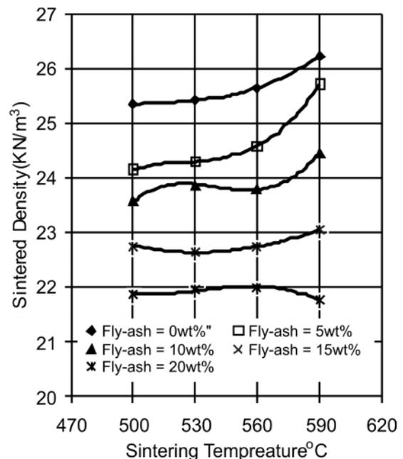
Figure 13: Effect of Sintering Temperature on Sintered Density of Al-15wt% Pb/fly-ash Composites Compacted at 300MPa
