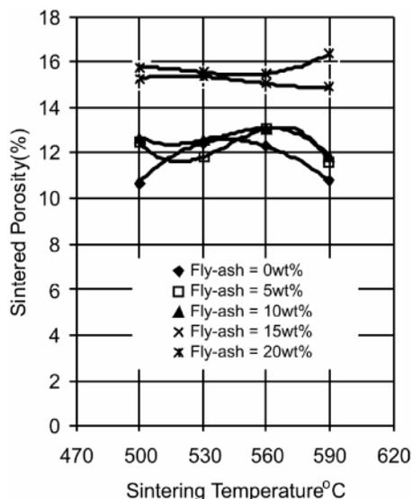
Figure 25: Effect of Sintering Temperature on Sintered Porosity of Al-15wt% Pb/fly-ash Composites Compacted at 400MPa
