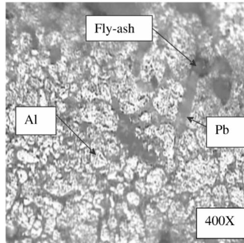
Figure 7: Microphotograph of Al-15wt% Pb/5wt% Fly-ash Composite Compacted at 400MPa and Sintered at 500 °C
