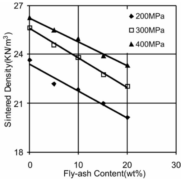
Figure 10: Effect of Fly-ash Content on Sintered Density for Al-15wt% Pb/fly-ash Composites Sintered at 560 °C
