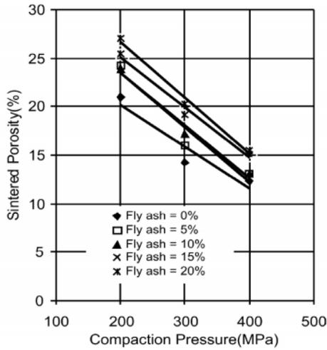
Figure 17: Effect of Compaction Pressure on Sintered Porosity of Al-15wt% Pb/fly-ash Composites Sintered at 560 °C
