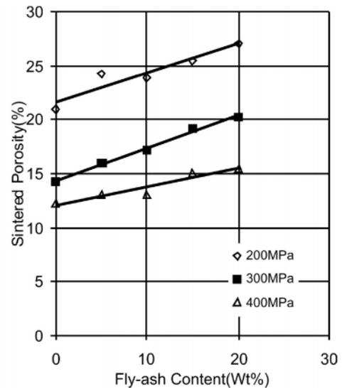
Figure 21: Effect of Fly-ash Content on Sintered Porosity of Al-15wt% Pb/fly-ash Composites Sintered at 560 °C
