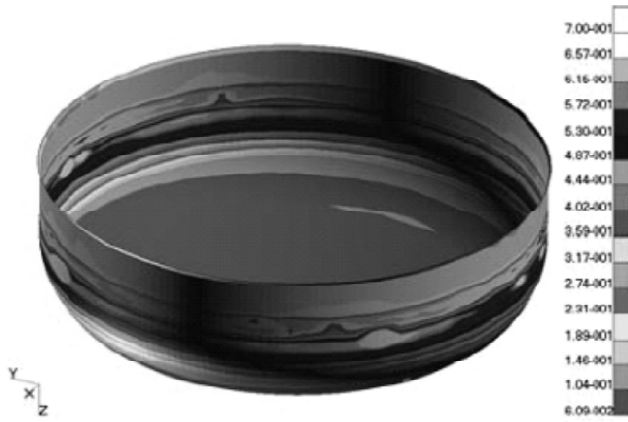
Figure 14: Total Equivalent Plastic Strain Distribution
