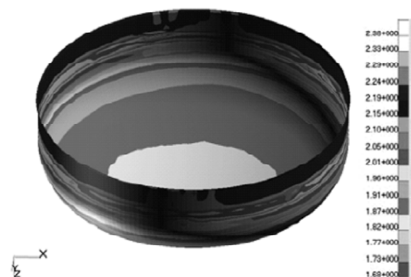
Figure 12: Thickness Distribution after Forming
