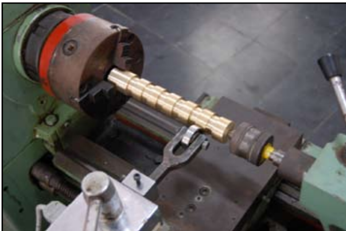
Fig. 9: Photograph Showing Close Up View of Experimental Set Up of Roller Burnishing Process on Lathe
