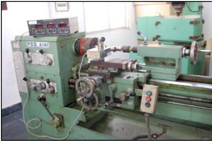
Fig. 8: Photograph of Experimental Set Up of Roller Burnishing Process on Lathe With Brass Work Piece
