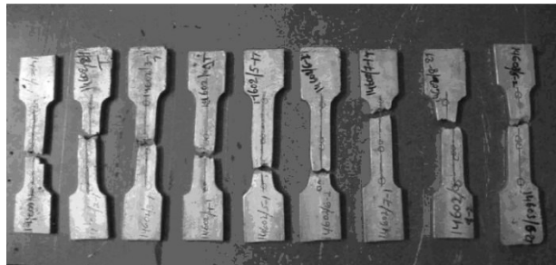
Figure 3: Tested tensile Al/SiC Composite specimens
