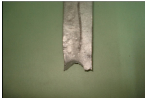
Figure 11: SEM tensile fracture surface of the 12% V_f Al/SiC composite
