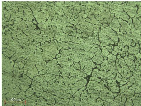
Figure 5: Microstructure of MMC (Al 7072 matrix, 16% Al<sub>2</sub>O<sub>3</sub>, 10µm particle size), 200X
