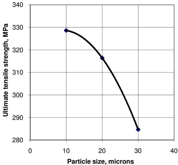
Figure 8: Influence of particle size on the ultimate tensile strength of Al/ Al<sub>2</sub>O<sub>3</sub> composite
