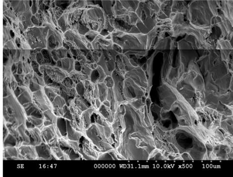
Figure 11: SEM of fracture surface of  $\text{Al}_2\text{O}_3/\text{Al6063}$  composite ( $V=20\%$  and  $P=10\mu\text{m}$ ); 1000X
