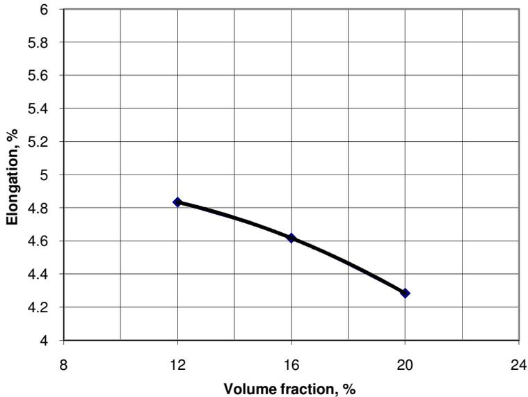
Figure 7: Influence of volume fraction on the ductility of Al/ Al<sub>2</sub>O<sub>3</sub> composite
