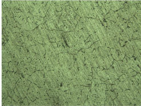
Figure 3: Microstructure of MMC (Al 6061 matrix, 12% Al<sub>2</sub>O<sub>3</sub>, 10µm particle size), 200X
