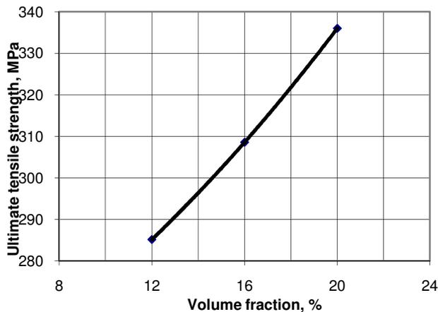
Figure 6: Influence of volume fraction on the ultimate tensile strength of Al/  $\text{Al}_2\text{O}_3$  composite
