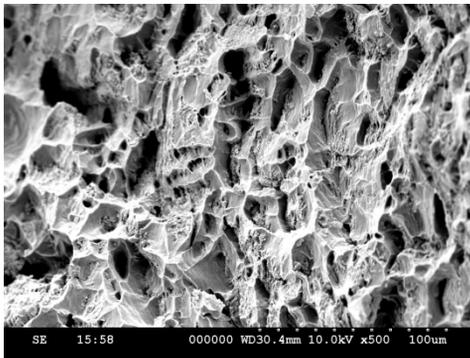
Figure 12: SEM of fracture surface of  $\text{Al}_2\text{O}_3/\text{Al7072}$  composite ( $V = 6\%$  and  $P = 10\mu\text{m}$ ); 1000X
