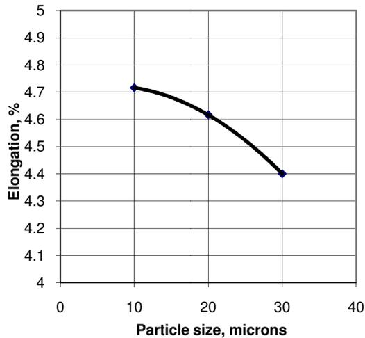
Figure 9: Influence of particle size on the ductility of Al/ Al<sub>2</sub>O<sub>3</sub> composite
