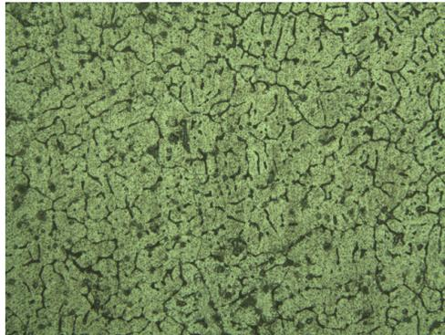
Figure 4: Microstructure of MMC (Al 6063 matrix, 20% Al<sub>2</sub>O<sub>3</sub>, 10µm particle size), 200X
