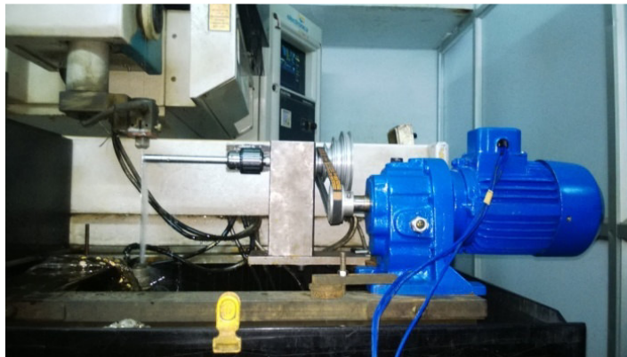
Figure 1: The experimental setup of turning with wire EDM
