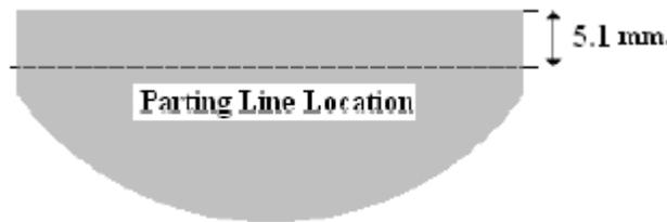
Figure 3: Parting line location on the forged part
