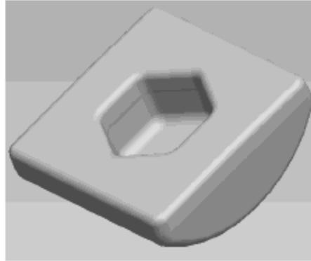
Figure 2: Solid modeling of the forging
