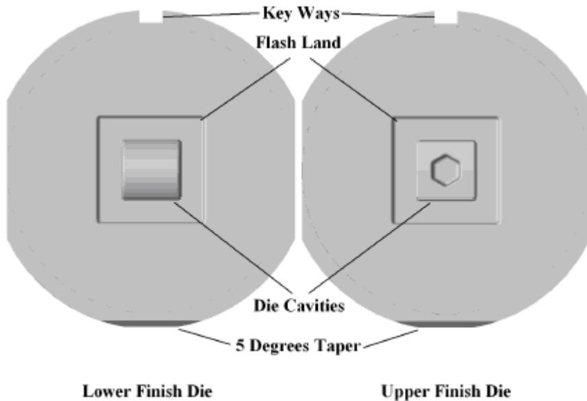
Figure 6: Lower and upper finish dies
