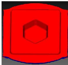
Figure 10: Die filling during forging operation.
