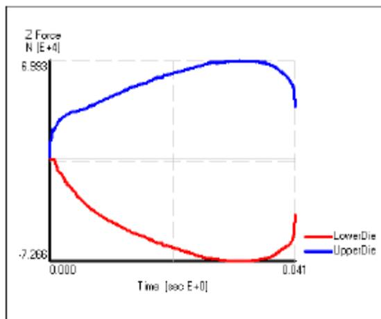
Figure 11: Die force for upsetting operation.
