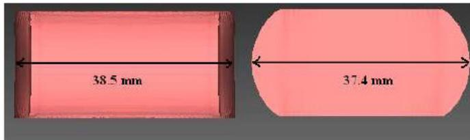
Figure 9: Dimensions of billet after forging operation.
