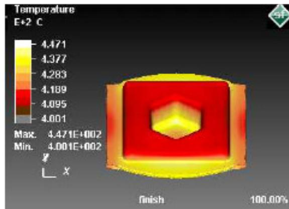
Figure 16: Temperature distribution for finish operation of at 400 °C
