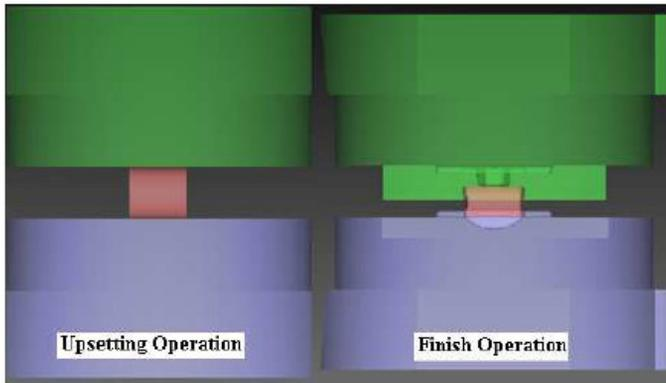
Figure 8: Position of billet on the upsetting die and finish die.
