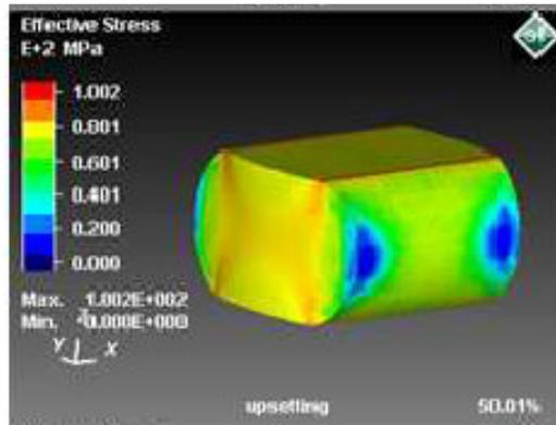
Figure 13: Maximum stress distribution for the upsetting operation at 400 °C
