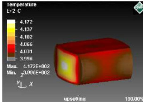
Figure 15: Temperature distribution for upsetting operation at 400 °C
