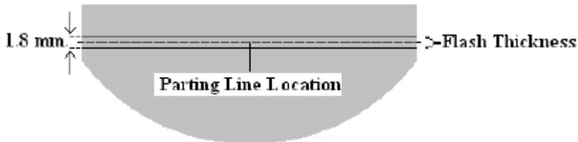
Figure 4: Flash thickness on the forged part
