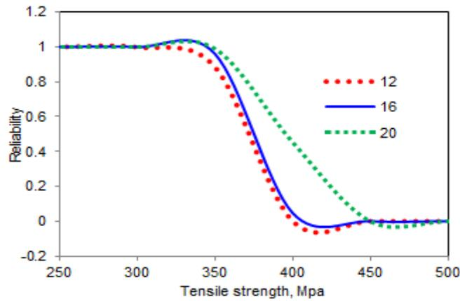
Figure 14: Reliability Graphs for Tensile Strength of 7020/SiC<sub>p</sub>
