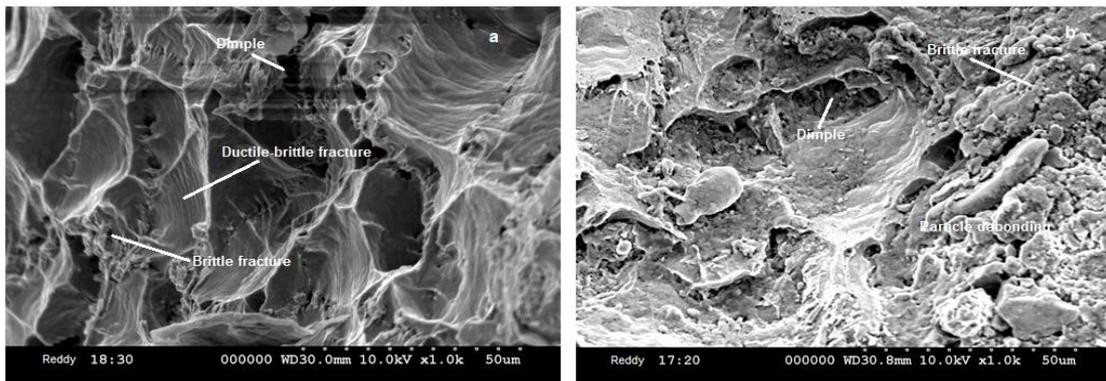
Figure 15: SEM of Fracture Surface of 7020/SiC Composites (a) of 20% V<sub>p</sub> and 800nm Particle Size (b) of 20% V<sub>p</sub> and 20 μm Particle Size
