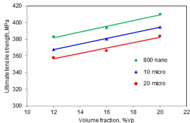
**Figure 3: Variation of the Tensile Strength with the Volume Fraction and Particle Size of SiCp**
