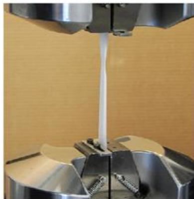
**Figure 2: Tensile Testing of Metal Matrix Composite**
