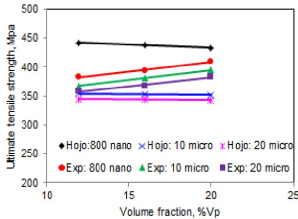
Figure 11: Comparison of Hojo Criterion with Experimental Values
