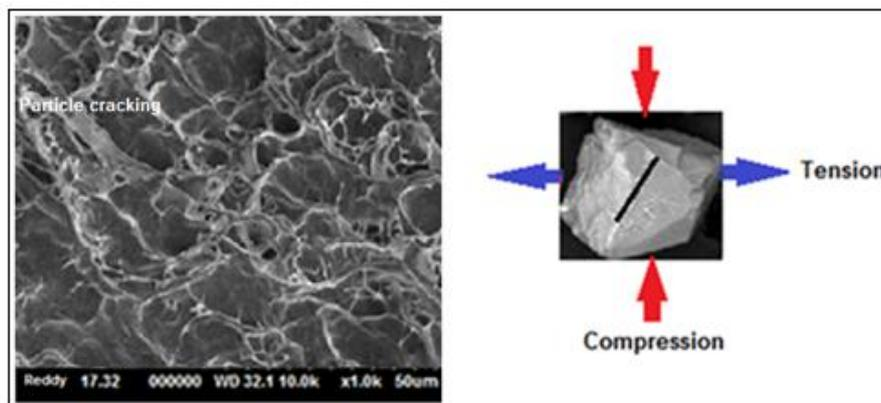
Figure 6: Particle Cracking due to Tensile Loading
