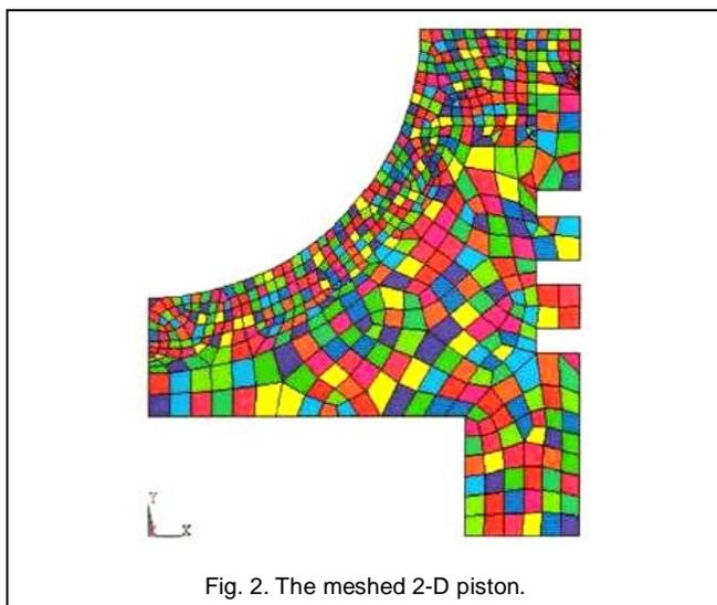
Fig. 2. The meshed 2-D piston.
