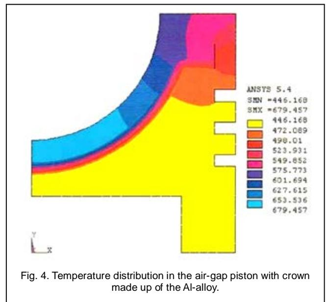
Fig. 4. Temperature distribution in the air-gap piston with crown made up of the Al-alloy.
