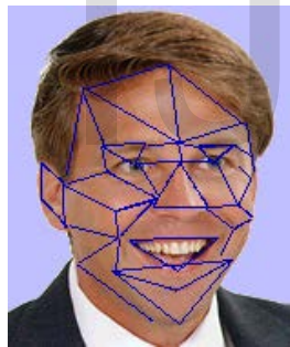
Fig 4.1: Fiducial points such as starting and end points of eyebrow, eye pupil, tip and side points of nose, two end points of mouth and tip of chin etc., and the edges joining these points.
