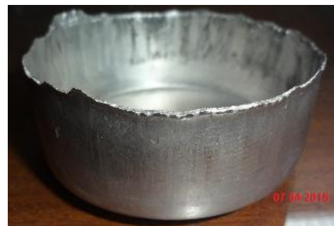
Figure 24: The successful deep drawn cup
