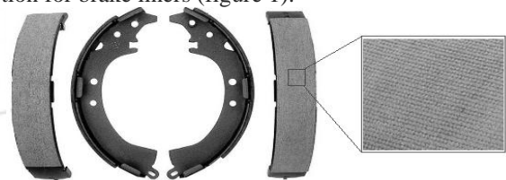
Figure 1: Goal of the present work to fabricate Kevlar 49 (Woven type)/epoxy composite for brake liners.
