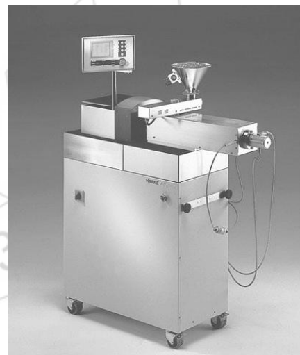
Figure 1: Torque rheometer with a twin-rotary mixer
