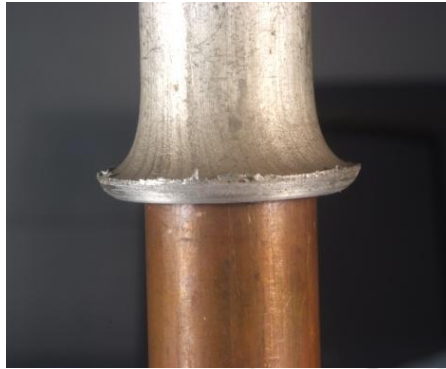
Figure 14: Welding aluminum and brass with trial 7 conditions.
