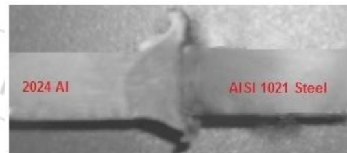
Figure 17: Welding 2024 Al alloy and AISI 1021 steel with trial 7 conditions
