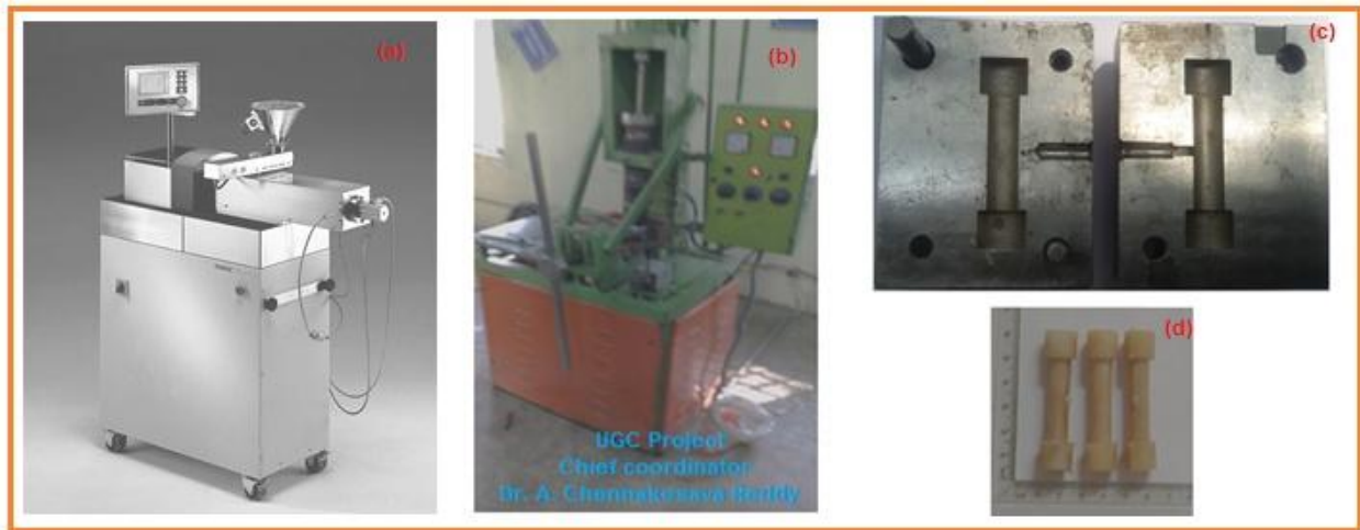
Figure 1: Preparation of test samples: (a) Torque rheometer with a twin-rotary mixer, (b) Injection molding machine and (c) Two mold halves and test specimens.
