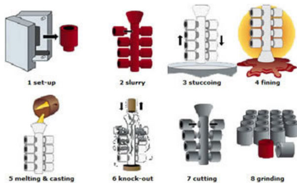
Figure 2. Fabrication investments shells and casting of 7075 aluminum alloy.
