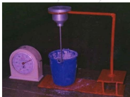
Figure 2: Measurement viscosity of investment slurry.
