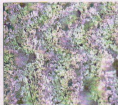
Fig. 5 Microstructure of Al-15% Pb-10% Fly Ash at 300 MPa
