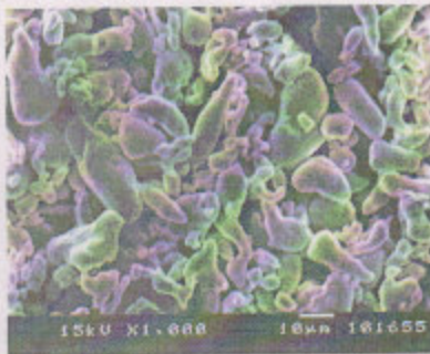
Fig. 1 SEM Photograph of Aluminum Powder
