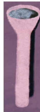
Figure 2: Alumina investment shell mould.
