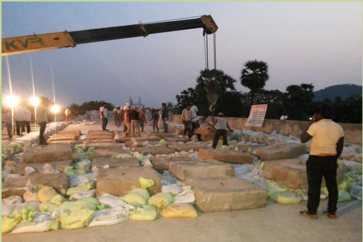
ICS Work : Load testing setup arranged for High level bridge at Bhimavaram
