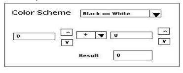
The Color Scheme may be Black on White or Blue on Yellow (selectable) and accordingly all components colors must be changed. The values can be either entered or increased or decreased by a step of 10. The operators are +, -, / and \* (selectable). Once any change takes place, the result
