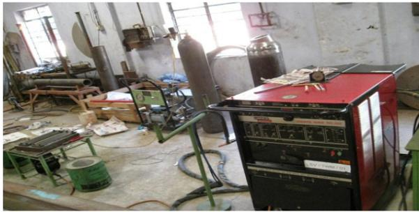
Figure 3: Lincoln Electrical square wave TIG 355 M/C
