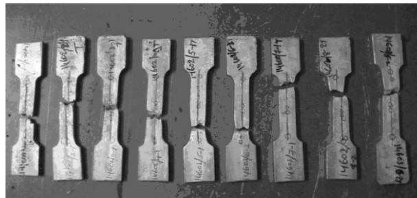
Figure 3: Tested tensile Al/SiC Composite specimens
