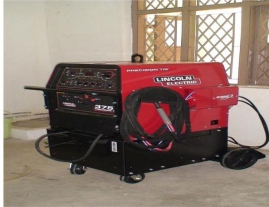
Figure1: Precision TIG 375-TIG welding machine
