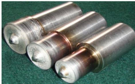
Figure 2: Taper cylindrical pin profiles
