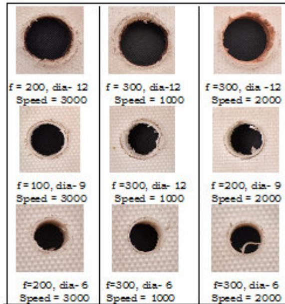
Figure 3: Typical drilled holes observed at different drilling condition
