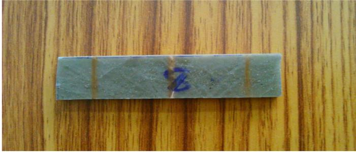
Figure 3: Three point bend test specimen
