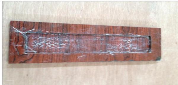
Figure 1: Mould for preparation of composite specimen
