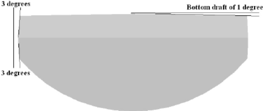
Figure 5: Draft angle on the forged part
