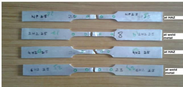
Figure 4: Tensile test specimens after test(1.5&2.5mm thick)
