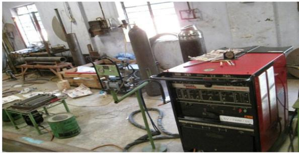
Figure 3: Lincoln Electrical square wave TIG 355 M/C
