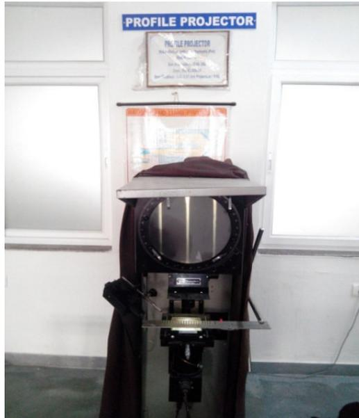
Figure 5: Profile projector with work piece to measure kerf width
