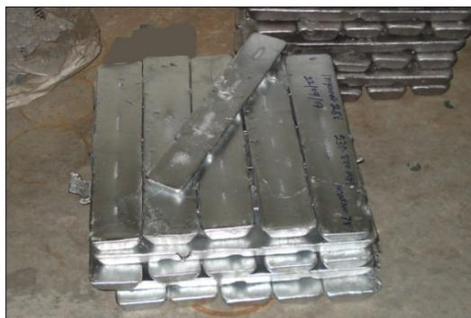
Figure 1: Aluminum 6061 alloy ingots
