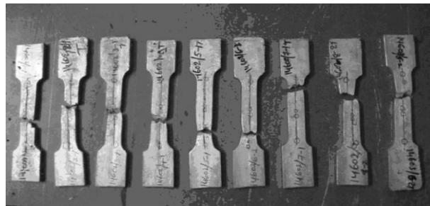
Figure 3: Tested tensile Al/SiC Composite specimens
