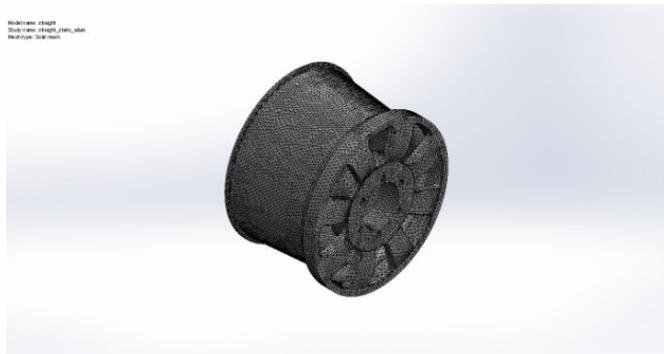
Figure 2: meshed component for straight cross member
