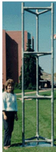
Figure 3. P100/AZ91C Gr/Mg tubes produced by the vacuum-assist casting process: (a-left) as-cast tubes, and (b-right) demonstration Gr/Mg truss structure.
