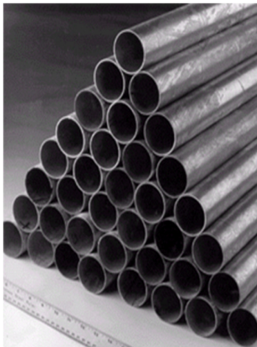
Figure 3. P100/AZ91C Gr/Mg tubes produced by the vacuum-assist casting process: (a-left) as-cast tubes, and (b-right) demonstration Gr/Mg truss structure.
