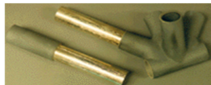
Figure 4. Cast SiC p /Al attachment fittings: (a-top) multi-inlet fitting for a truss node, and (b-bottom) cast fitting brazed to a Gr/Al tube.
